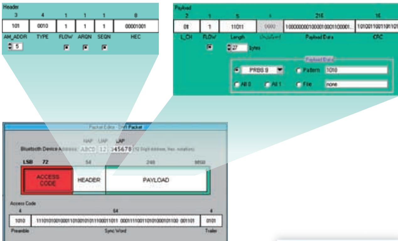
FIG 3 The packet editor configuration panel makes it very easy and convenient to configure data packets tailored to user's application
