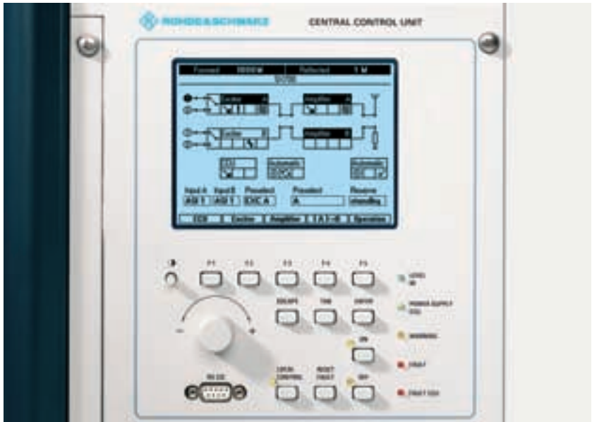
FIG 2 The transmitter is controlled via the user interface in the control panel of the Exciter SV700 or from an external PC
