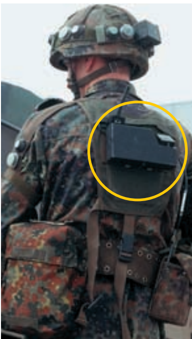
FIG 1 The compact and lightweight subscriber unit is usually mounted on the back
